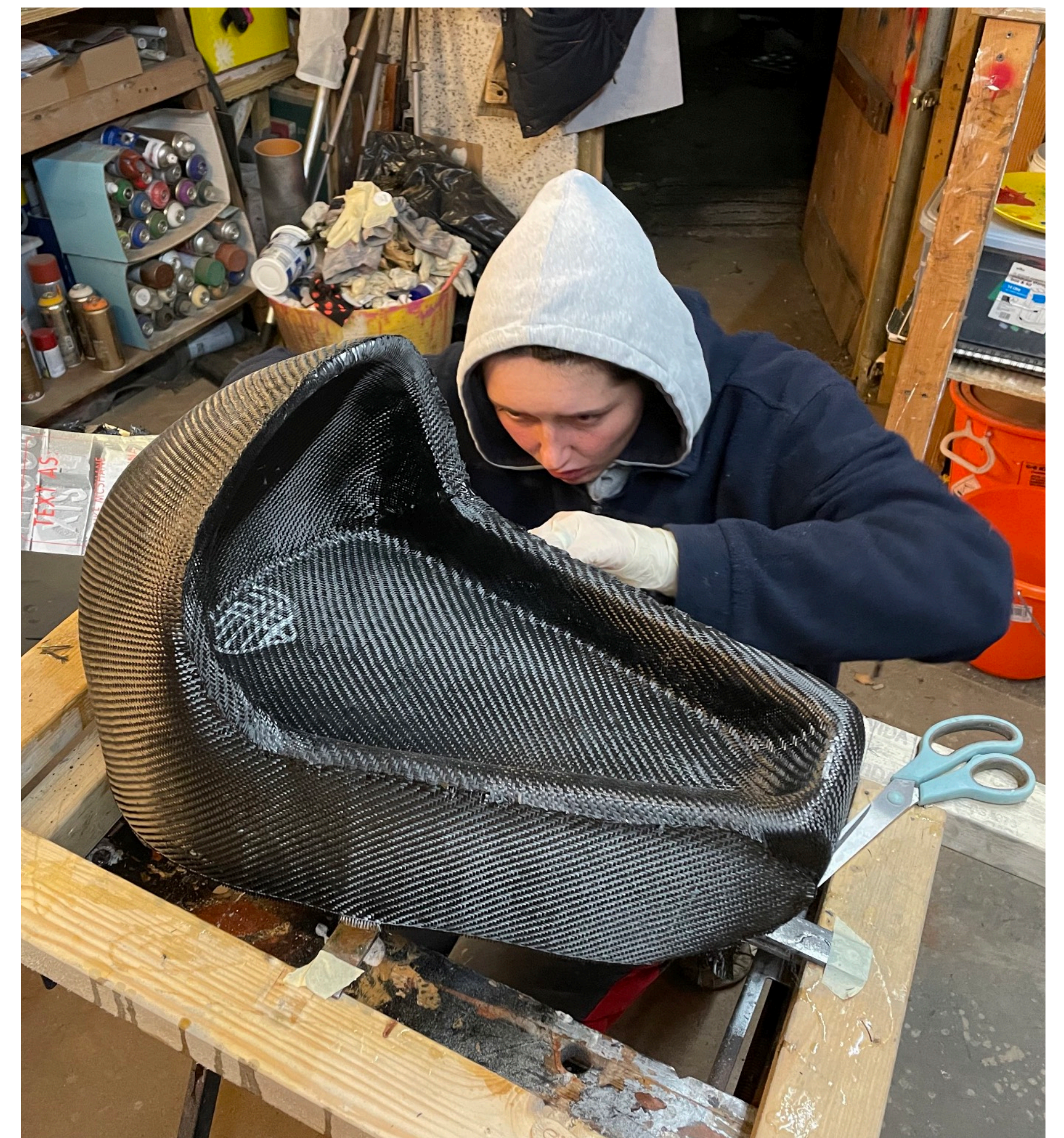
Design and fabrication of three different carbon fibre female urinal prototypes for Peequal (the first British female urinal company).
